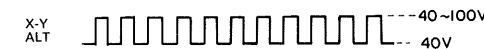
Fig. 31 Q4, Collector Signal A SWEEP TIME = B SWEEP TIME DELAY TIME MIN
